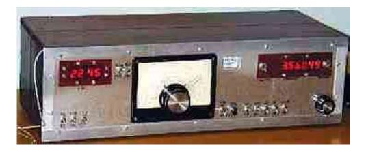
The defective digits were replaced (with some difficulty), and the display duty cycle changed to 1 in 8. This little clock is now fixed in the front panel of my <u>Polyphase receiver</u> exactly as intended. I usually set it to UTC (GMT) and use it for logging the start and end times of radio communications. The clock does not generate any detectable interference in the radio receiver. The battery backup does not function well: I think that battery needs replacing.
