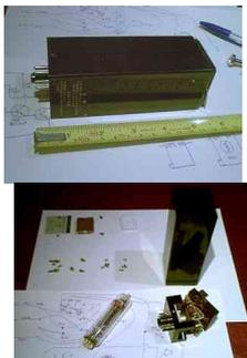
Here are some pictures of the OCXO. Left: assembled; Right: Disassembled! The unit was produced by Fujitsu Limited. It is very nicely engineered. Inside filling the crystal enclosure are a large quantity of tiny glass beads, a small number of which inevitably escaped onto my kitchen floor. That was a good enough excuse to sweep the floor, and it is believed that a high proportion were recovered from the resulting dust pile.
