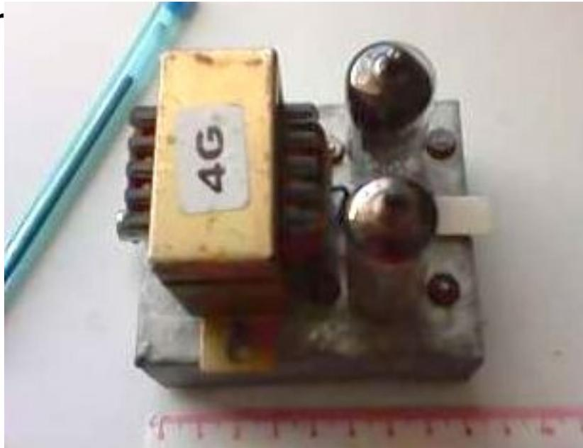
A simple QRP transceiver with full QSK for the CW sub-band of 40m. It uses two valves, a 6AQ5 pentode, and a 12AX7 double triode.
